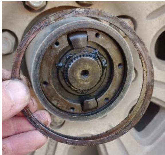
Remove (14) HubSnap Ring with flat screwdriver or pick
