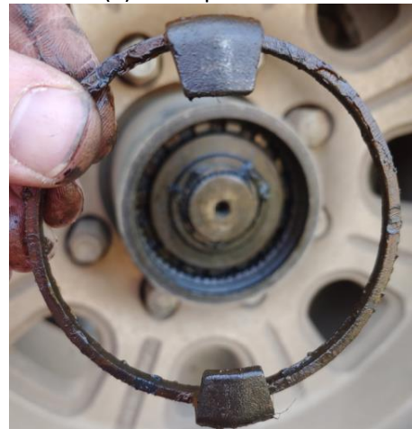
Remove (13) Axle Snap Ring with flat screwdriver or pick
