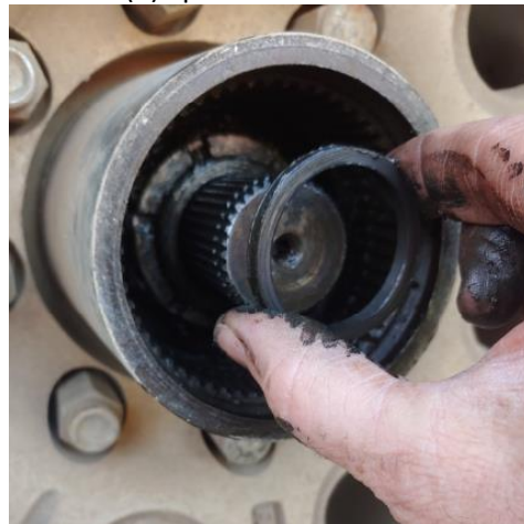
Remove 1 st Axle Nut with 2-5/8" OD 6-lug spindle nut socket
