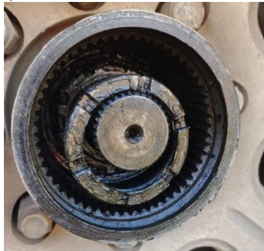
Remove 1 st Axle Nut with 2-5/8" OD 6-lug spindle nut socket
