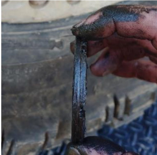
Remove Lock Ring (Teeth facing outward)
