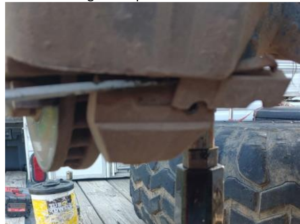
Remove Wedge with punch and hammer
