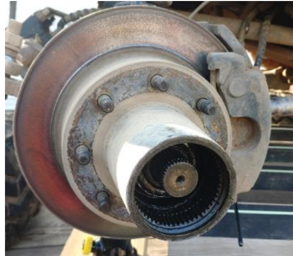
Remove caliper lock screw with 1/4" Allen
