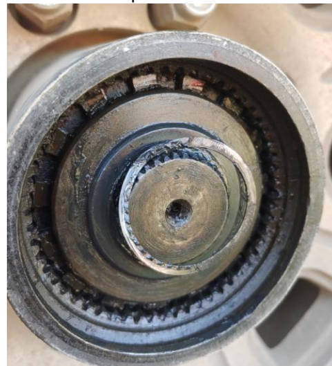
Remove (13) Axle Snap Ring with flat screwdriver or pick
