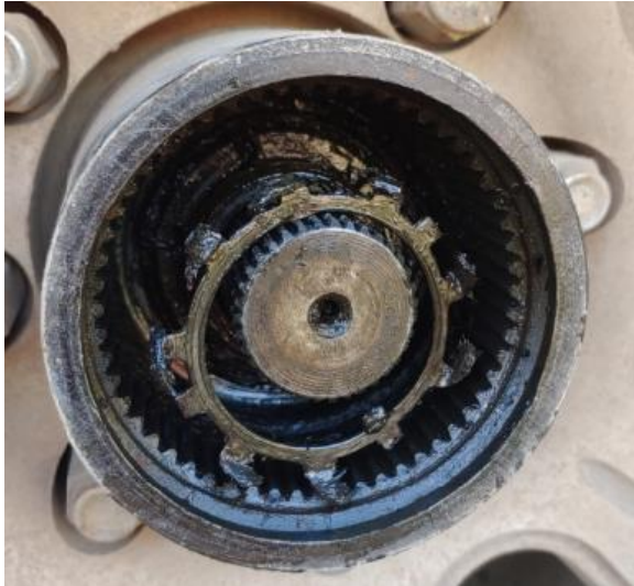
Remove Lock Ring (Teeth facing outward)
