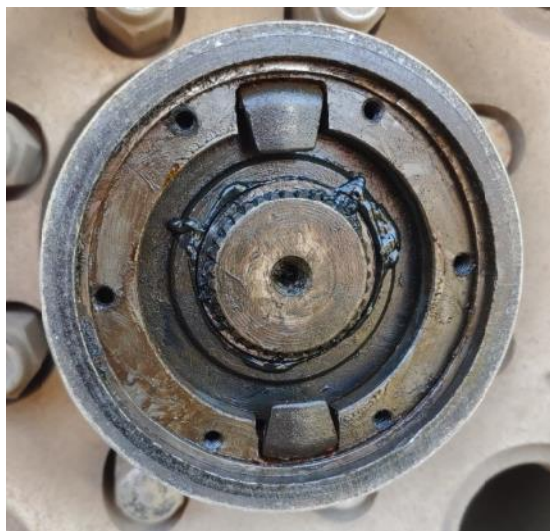
Remove (14) HubSnap Ring with flat screwdriver or pick
